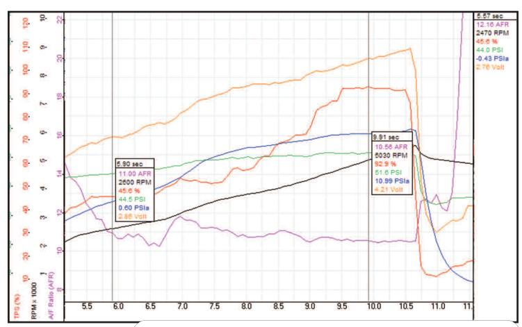
Using a laptop and Innovate's LogWorks software, you can datalog four channels via the PSN-1; nitrous bottle pressure, engine-RPM, air-fuel ratio, and nitrous solenoid activation state.
