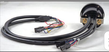
The back of the unit is sealed and consists of a group of pre-terminated leads for the various sensors, making it a truly easy, plug-and-play affair.
