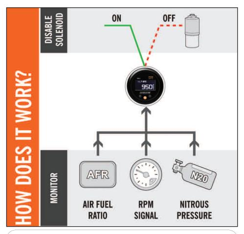
The PSN-1 continuously monitors your AFR and nitrous bottle pressure. As long as they are within the user-defined "safe range" and engine-RPM is within the specified range, the nitrous solenoid will be activated. Should any parameter fall below a threshold, the nitrous cuts off, keeping the engine safe.
